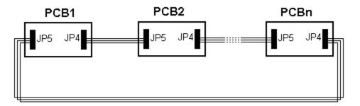
Note that we only need one PCB in the cascade connects to RS232 input from the rear connector because the interconnection of JP4 and JP5.
